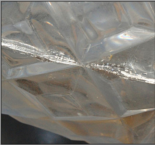
Adhesive bond Paraloid B72 in ethanol. Note bubbles in bond
