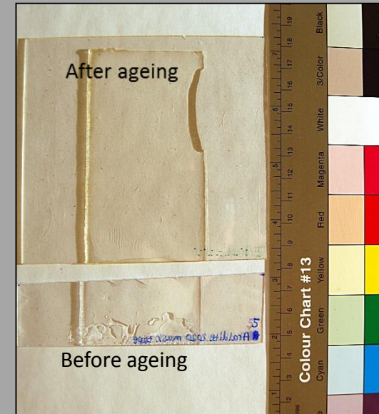
Araldite 2020 before and after (top) ageing on transparent polystyrene
