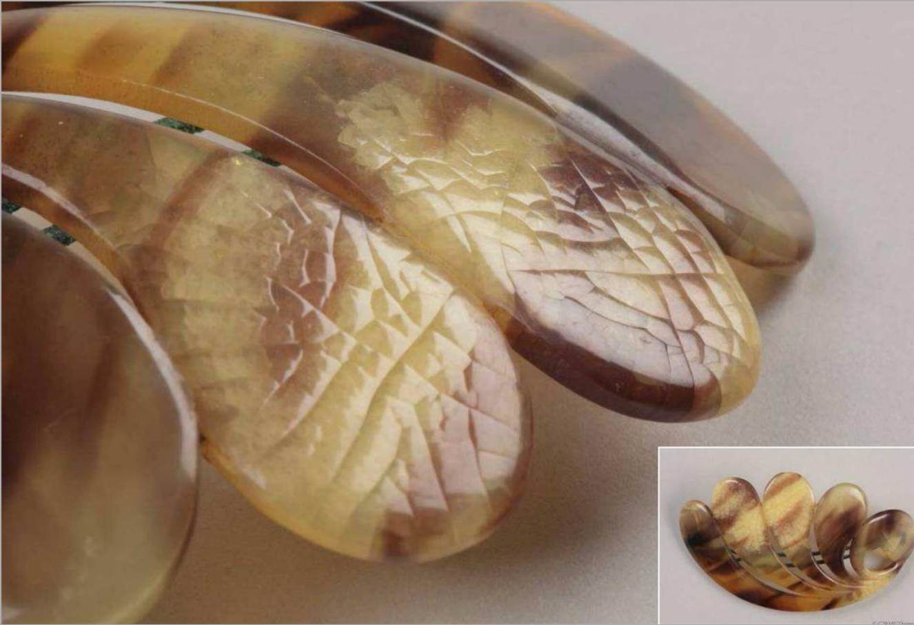
Krackelering (craze), hårkam cellulosanitrat. Damage atlas, POPArt
