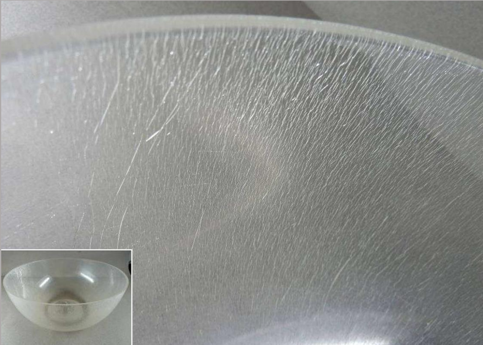
Krackelering , skål PMMA. Damage atlas, POPArt
