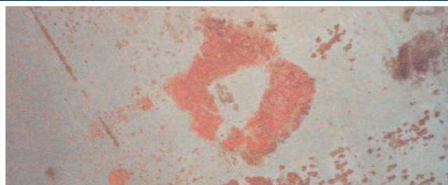
Figure 100. When objects are touched with bare hands, skin oils and fatty acids can be transferred onto the surface. These chemically active compounds react locally with the surface and form corrosion on polished metals and stains on porous surfaces. Sometimes, a handprint may be visible. Corrosion on metals because of fingerprints is, under normal conditions, visible after three to nine months.
