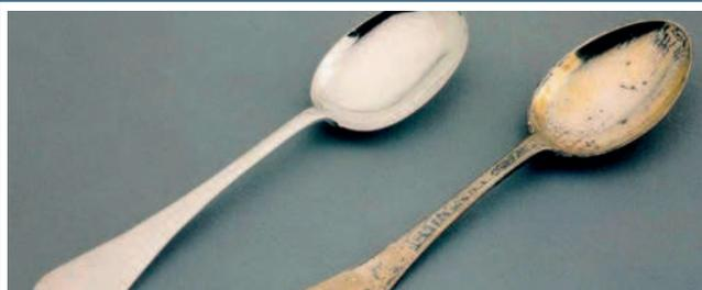
Figure 102. Silver objects tarnish and silver sulphide is formed. Because the concentrations of hydrogen sulphide ( $\text{H}_2\text{S}$ ) and carbonyl sulphide ( $\text{OCS}$ ) are very low and the reaction very fast, the reaction rate is completely determined by the speed at which the gases reach the surface. Under normal conditions, the first phase of tarnish, a pale-yellow surface, is visible in around six months to a year.
