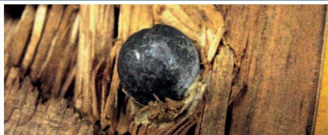
Figure 101. A lead musket ball was shot into a wooden board to study the penetration depth. The bullet has reacted locally to form lead carbonate. This is a good example of intrinsic contamination: the organic acid from the board reacts with the susceptible lead surface.
