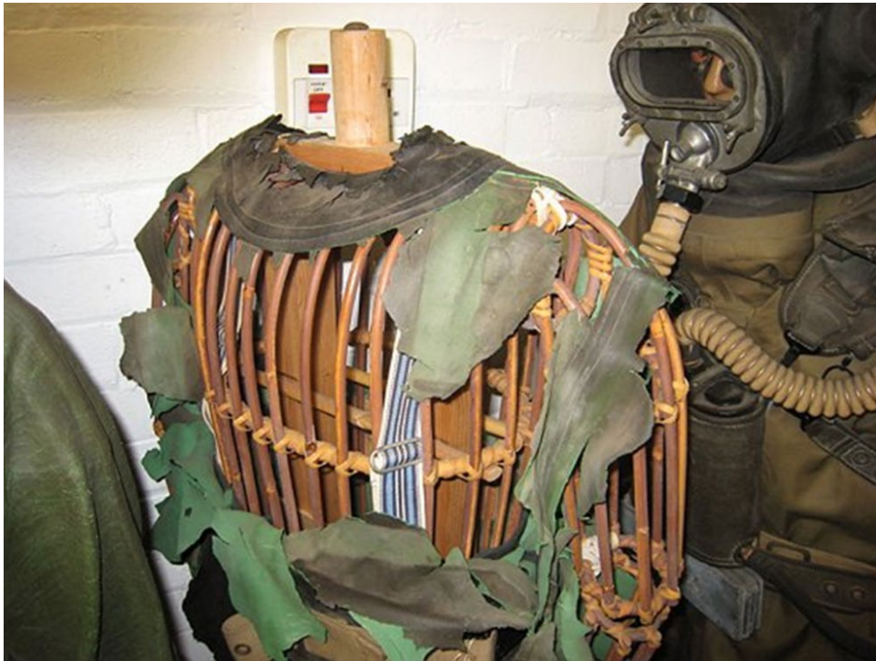
Figure 2. Modern materials are sensitive to chemical degradation by oxidation. Diving suit, Imperial War Museum, Duxford Airfield, UK. Photo: Poul Klenz Larsen.
